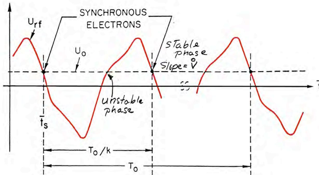
Particles change energy according to the phase of the field in the RF cavity
