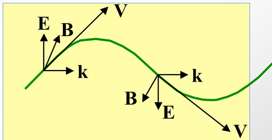
Electron trajectory through wiggler with two periods
