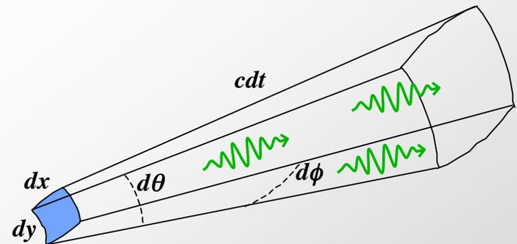
$$\text{Flux} = \frac{d\dot{N}}{d\lambda} = \int \text{Brightness } dS d\Omega$$
